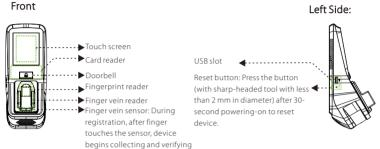
>>> Finger Vein Device fingerprint and finger vein.
