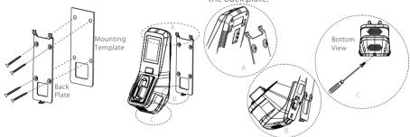
Note: For user heights between 150CM to 170CM, it is recommended to install the device at 140CM above ground (may be modified according to user average height).
