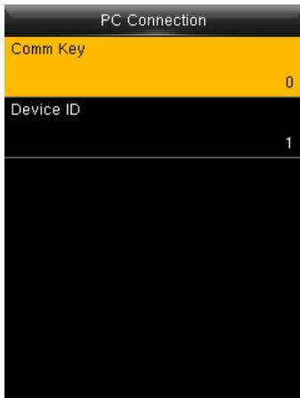
**Comm Key:** Set 1-6 digits connection password, the password must be input when PC software is to connect device to read data.
