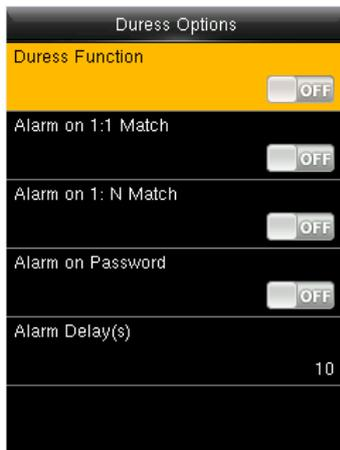
**Duress Function:** If enabled, a fingerprint or an ID number successful verification in 3 seconds after pressing help, The duress alarm will come out. Help can be set in keyboard.
