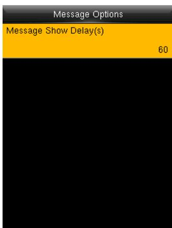
**Message Show Delay (s):** It means the duration that personal message shows. The personal message showing interface will back to initial interface after reaching Message Show Delay. The valid value is 1-99999 seconds.
