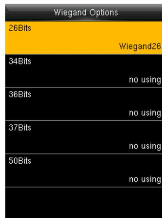
**Wiegand Format:** The system has five built-in formats: Wiegand 26-bits, Wiegand 34-bits, Wiegand 36-bits, Wiegand 37-bits and Wiegand 50-bits. Every format has two types of WiegandX and WiegandXa except for Wiegand 50-bits. You can select more than one wiegand formats.
