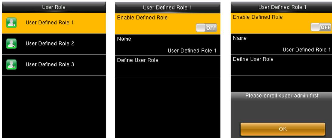
A Super admin must be enrolled before a new role is defined, or it can not be enabled.
