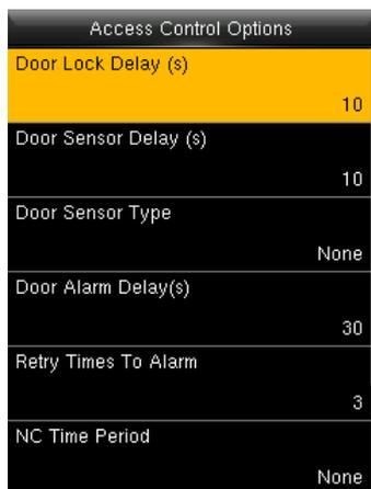
**Door Lock Delay(s):** The enabling time of electronic lock. The value ranges from 1 to 10 seconds.
