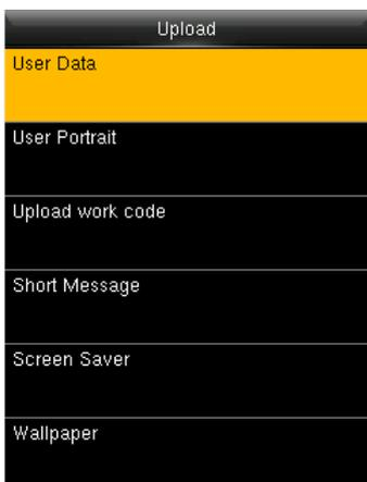
**User Data:** Upload user data saved in USB disk to the device.
